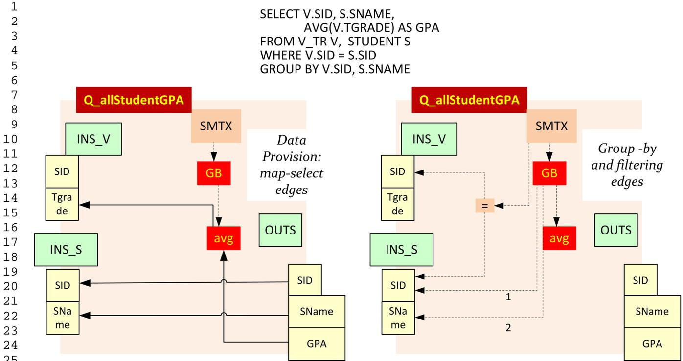
Fig. 5 The graph of a group-by query. To avoid confusion, we depict the edges in two snapshots of the graph: provider edges (left) and filtering and grouping edges (right).
