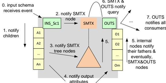
Figure 2. Protocol for the message propagation mechanism
