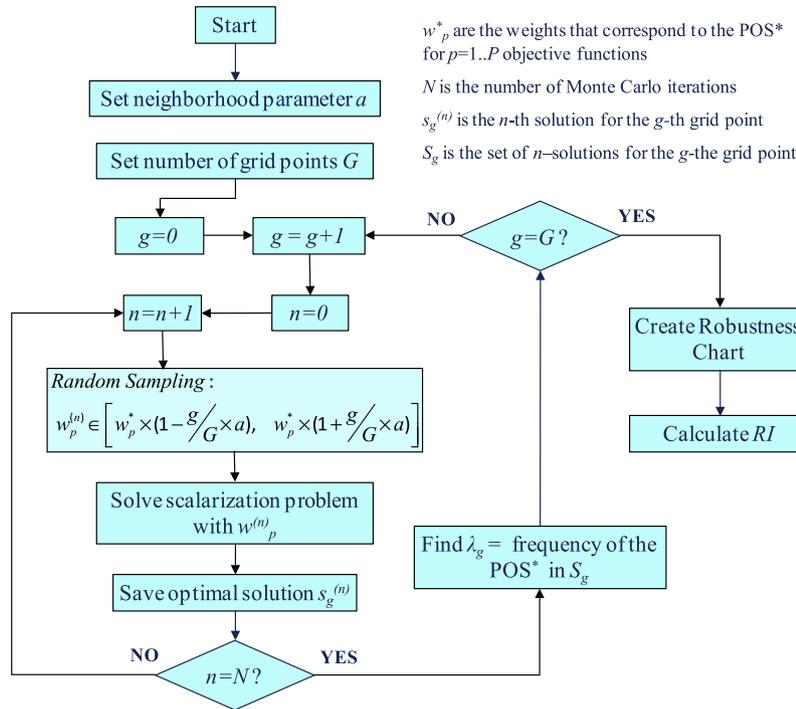
Fig. 3. Flowchart of the algorithm for robustness analysis in multi-objective programming.
