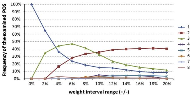
Fig. 5. Example of a joint Robustness Chart with  $F = 8$  Pareto optimal solutions.
