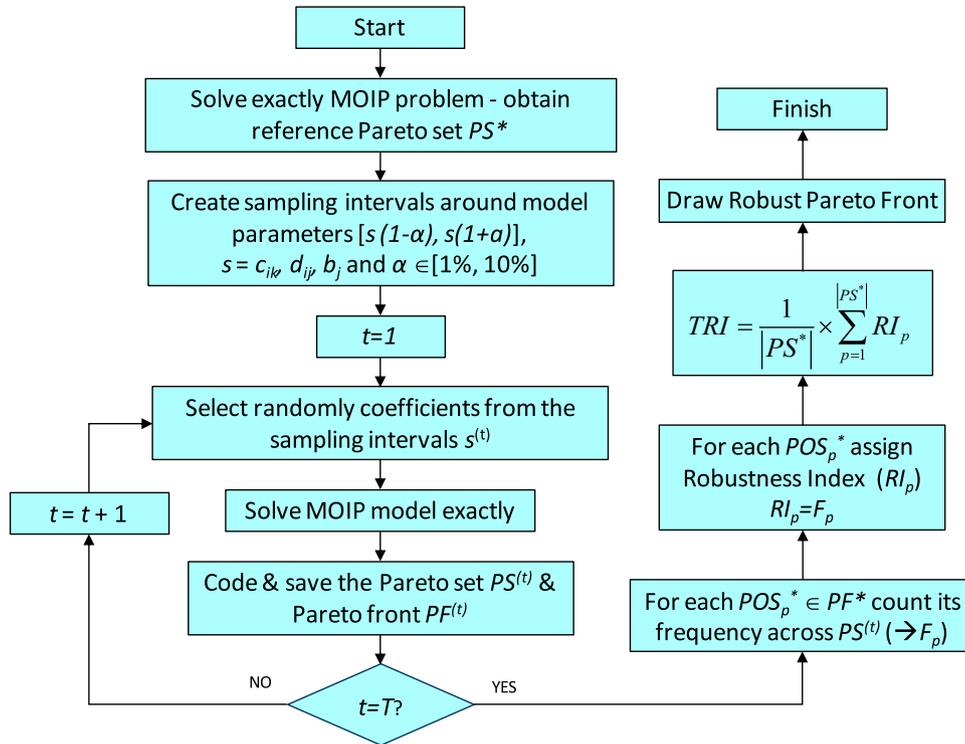
Fig. 2. The algorithm for estimating robustness in MOIP problems.
